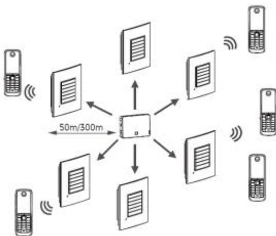
The maximum number of handsets that can be registered to your base station is not affected by the repeater. The repeater can be used to extend the coverage range in all directions, allowing several floors to be covered.
