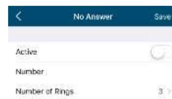
The App will offer the option to set this parameter up to 20 rings but Horizon only supports a maximum of 7 rings before diverting the call. If a number higher than 7 is selected, you will receive this error message.
