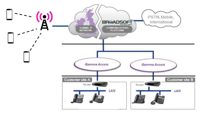
The main components are the Access Network, both fixed and mobile, the Gamma IP Network where the Communication Platform sits and the Customer Site which can be multiple as in this example.
